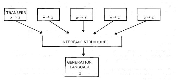
The output from the transfer components is, again, an interface structure which will, for each language, be input to one and only are generation component.
